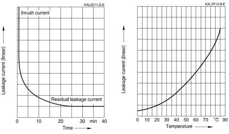
Figure 15 Leakage current versus time for which a voltage is applied
