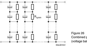
Figure 26 Combined parallel / series connection (voltage balancing by shunt resistors)
