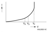
Figure 17 Voltage dependence of the leakage current
