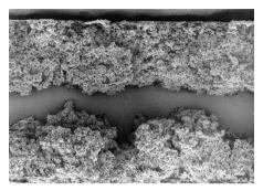
Figure 3 Anode foil for low-voltage capacitors (magnification 400x)
