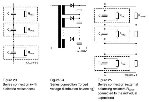
Experience has shown that it is preferable to choose balancing resistance values that will cause a current of approximately 20 times the leakage current of the capacitor to flow through the resistors. The equation for calculating the resistance value is:
