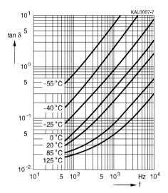
Figure 11 Low-voltage electrolytic capacitor "SIKOREL 125" (Example: 220 μF/40 V DC)
