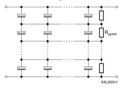
Figure 27 Combined parallel / series connection (group voltage balancing)
