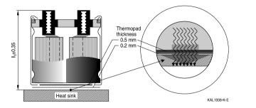
Figure 19 Heat sink mounting for capacitors with screw terminals
