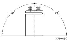
Figure 30 Recommended range of mounting positions
