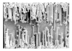
Figure 2 Anode foil for high-voltage capacitors (magnification 400x)
